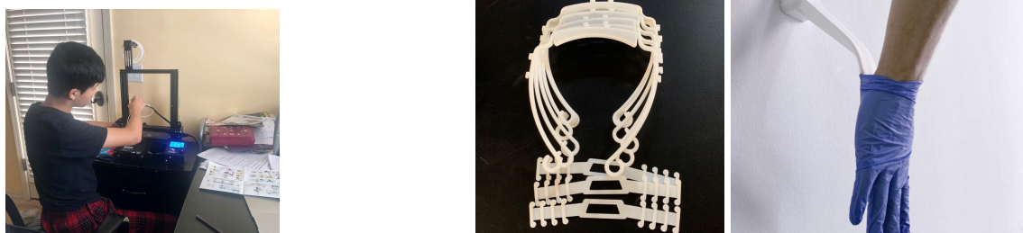
Phoenix Branch members work with a 3D printer (left) to produce face shield frames (center) and glove removal devices (right).
